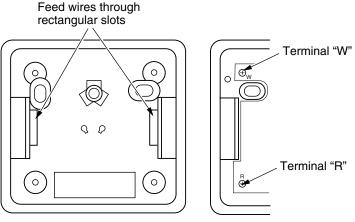
Figure 46 - Back View of Thermostat Base
